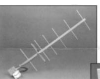
maximized at 11.0 dBd at the design frequency of 402 MHz which gave a narrow band width (394particular GOES application.
