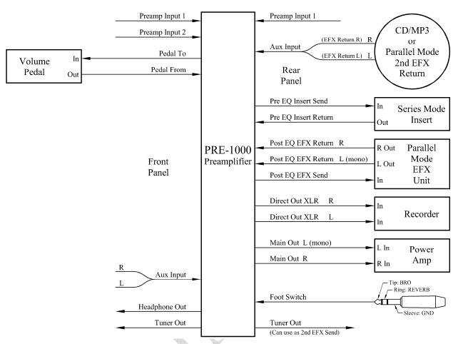
NOTE: Aux In L & R are on a 1/4 in TRS jack: Tip is Left, Ring is Right, Sleeve is Ground
